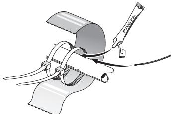
Install the temperature sensor with cable ties with the heat conducting paste and aluminium tape. Then insulate with supplied insulation tape.
