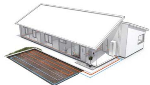
Surface soil – using a surface collector
