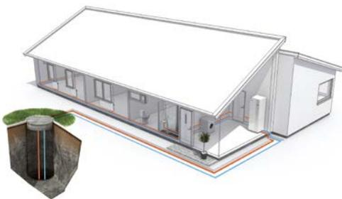
Rock – using a ground probe
